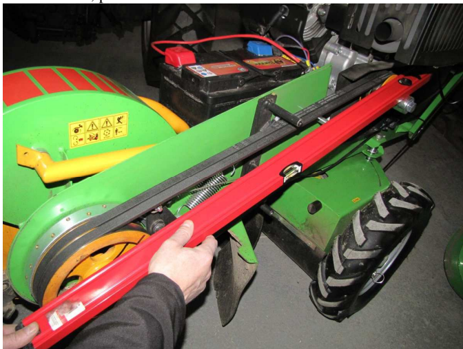
Alignment setting on the engine pulley
